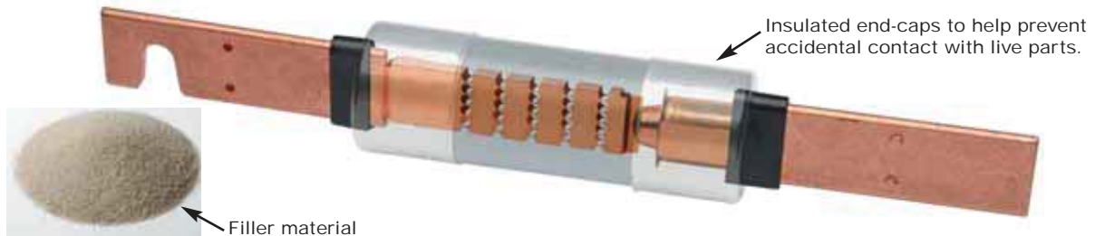
Figure 6. This is the LPS-RK100SP, a 100A, 600V Low-Peak, Class RK1, Dual-Element Fuse that has excellent time-delay, excellent current-limitation and a 300,000A interrupting rating. Artistic liberty is taken to illustrate the internal portion of this fuse. The real fuse has a non-transparent tube and special small granular, arc-quenching material completely filling the internal space.
