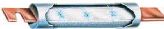
Figure 4. When subjected to a short-circuit current, several sections of the fuse link melt almost instantly.
