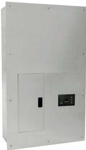
Controlled isolated power panels from Schneider Electric are designed to provide power for portable equipment outlets. In the past, most equipment operated on 60 A circuits. Today, these loads vary from 20 to 60 A and multiple pieces of equipment are being used. By applying the proper kVA loading, a panel can now provide power to multiple rooms and maintain safe operating conditions. All these panels are available in both one-phase and three-phase configurations with 5 to 25 kVA ratings.
