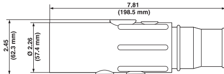
Ball Nose In-line Latching Male Connectors - Crimped
