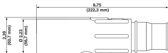
Taper Nose In-line Latching Male Connectors - Crimped
