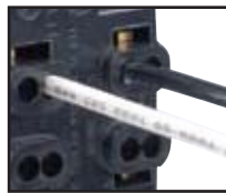
Quickwire™ Connection Insert wire into wire well. Wire is automatically clamped by spring action, insuring good electrical connection. For copper conductors only.
