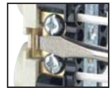
Two-Circuit Conversion To power each outlet of a duplex receptacle separately, simply break off the tab between the two terminals.
