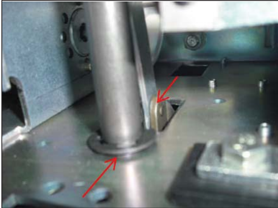
Figure 18: Lubricate with Klüber Unimoly GL 82 (continued)
