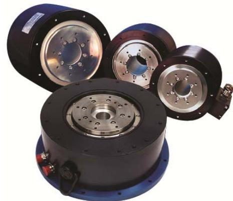
[Kollmorgen Housed Direct Drive Rotary \(DDR\)](#) motors offer high performance and zero maintenance in a precision servo solution. These motors combine large diameter, short length and a high number of magnetic poles to provide outstanding torque density, while eliminating the need for gearboxes, timing belts and other transmission components.
